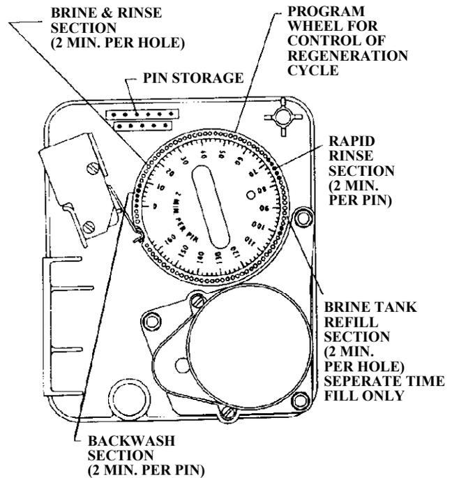
To change the length of refill time, move the two pins at the end of second group of holes as required.
