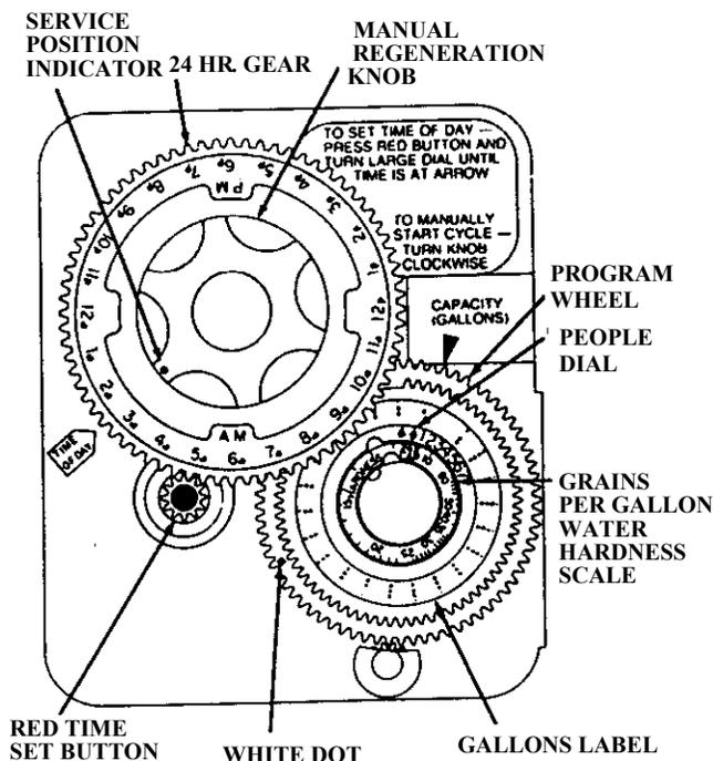
The black center knob will make one revolution in the following approximately three hours and stop in the position shown in the drawing.
